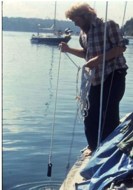
Figure 16 – Soundings with a lead line. This works. While somewhat tedious, combined with a hand-held GPS monitor, a representative understanding of the bathymetry can be achieved
