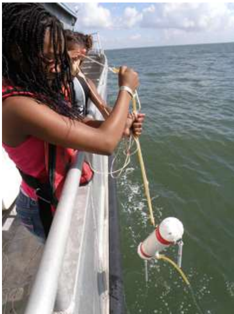
Figure 21 – Niskin bottle sampler Source NOAA National Marine Sanctuaries Source: http://flowergarden.noaa.gov/image_library/nabsyes2013images.html , and http://www.kc-denmark.dk .
