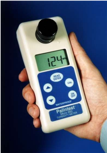
Figure 28 – Hand-held turbidity meter using water samples. 0.01 to 1000 NTU, 2 to 3% accuracy Source: http://www.camlab.co.uk/palintest-micro-950-turbidity-meter-p26036.aspx .
