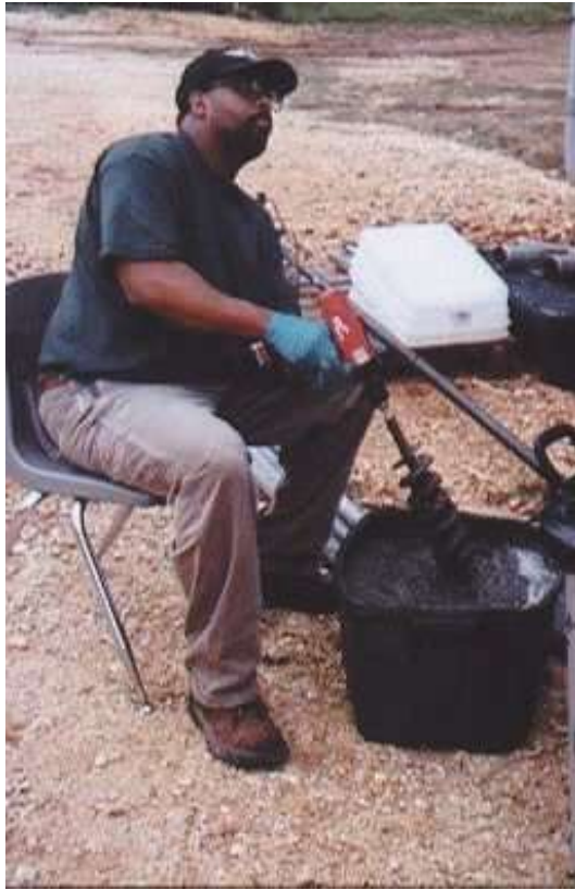
Figure A3-3 – Homogenizing a composited sediment sample using a mechanical mixer Photo by Chris Ingersol.
