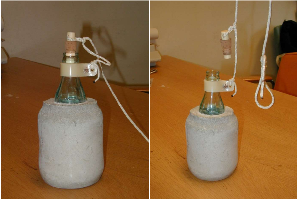
Figure 20 – Cola water sample in the locked position and once released Source: DHI, Denmark.
