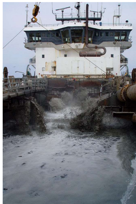
Figure 7 – On the left, a mechanical bucket dredging showing consolidated material, and on the right, the hopper of a dredge showing a slurry of dredged material Sources: Norfolk Dredging Inc. and Seaturtle.org.
