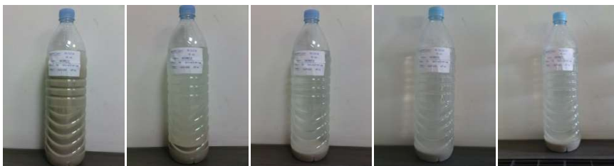
Figure 30 – A simple way of measuring percentage of fines
