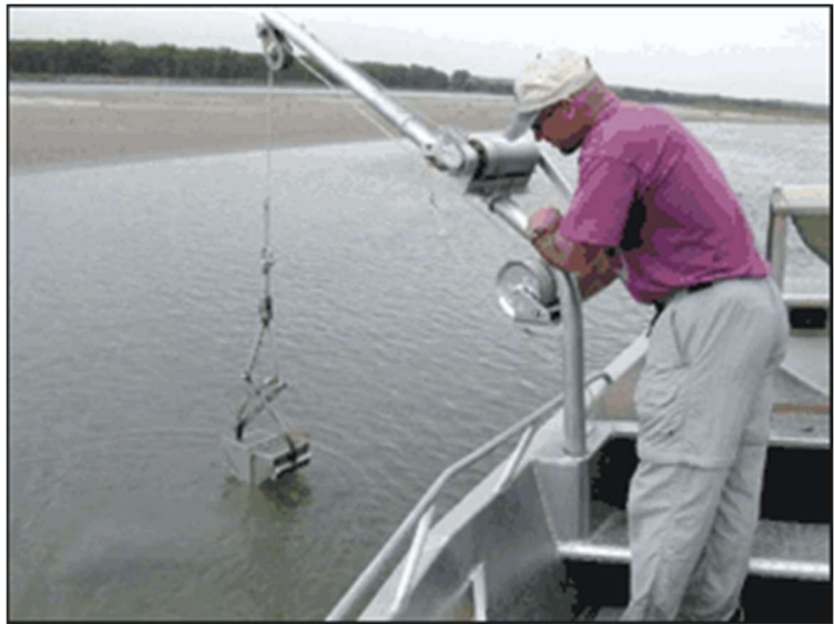
Figure 6 – Grab sampling sediments to assess extent of dispersion of sediments from the dump-site Source: http://infolink.cr.usgs.gov/Science/EMAP/index.htm .
