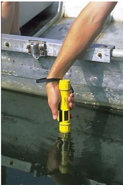
Figure 17 – Portable depth sounder. This Hondex Remote Portable Depth Sounder quickly determines water depth for sampling and depth studies. A transducer transmits high frequency pulses that reflect off the bottom and back to the unit where they are processed to determine depth. Depth range of 1.8 feet (0.5 m) to 240 feet (74 m). Cost US$259
