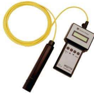
Figure 29 – Hand-held turbidity meter for in-water measurement. Range: 0.50 NTU to 1000 NTU Accuracy: + 5% Source: ENVCO website: http://www.envcoglobal.com/catalog/product/other-handhelds/wq770-handheld-turbidity-meter.html .
