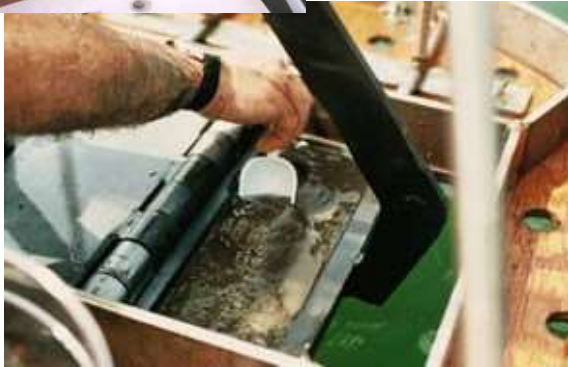
Figure 40 – Taking subsamples from a Ted Young modified Van Veen sampler
