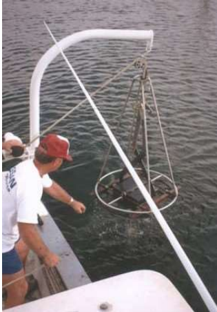
Figure 38 – Sampling using a Ted Young modified Van Veen sampler. Large grab samplers such as these require winches and sufficient boat size for efficient operation
