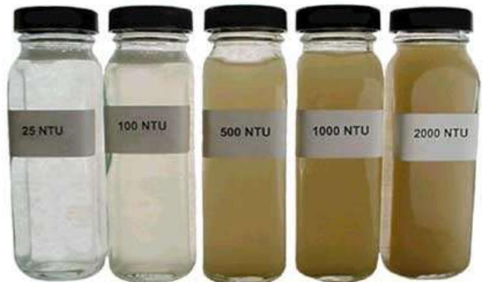
Figure 24 – Turbidity from 25 to 2000 NTU
